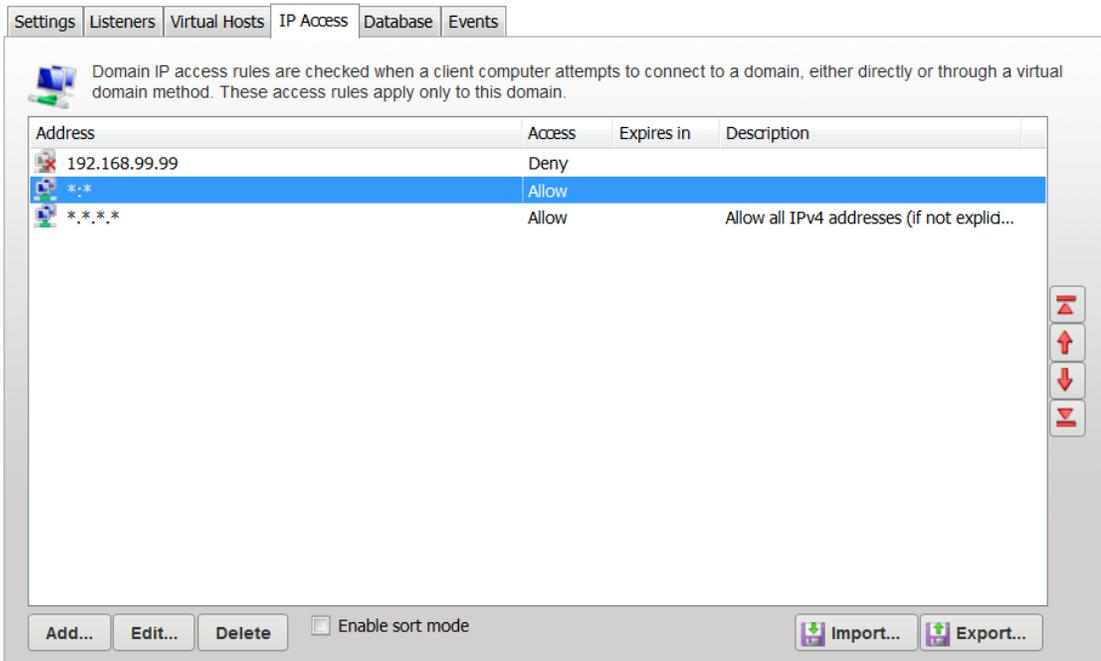
Domain IP access rules are checked when a client computer attempts to connect to a domain, either directly or through a virtual domain method. These access rules apply only to this domain.
